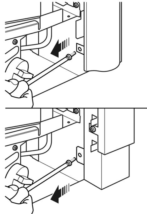
Figure 48. Removing the surround fixing screws
