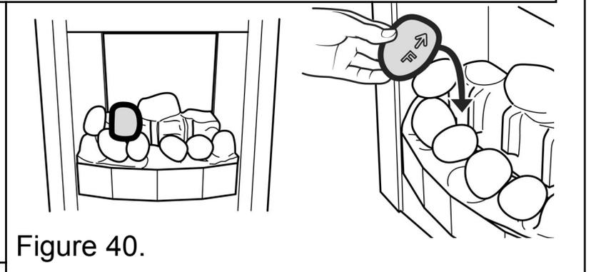
10. Hold pebble 'G' upright with the arrow pointing to the top. Place pebble 'G' between the front and rear base pebbles. It should rest on top of pebble 'B' & 'C' and rest against the moulded pebble in the rear pebble base. (See figure 41).
