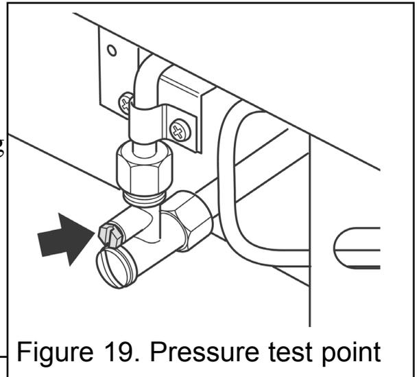
Figure 19. Pressure test point
